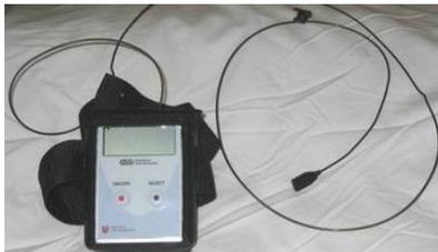
FIGURE 3: Dosimeter (Educational Direct Dosimeter, Unfors Instruments, Billdall Sweden)
