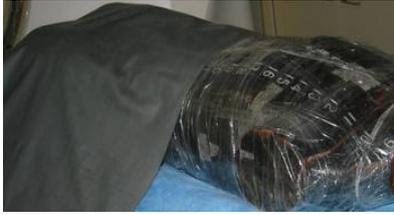
FIGURE 5: One layer of shielding wrapped 180° around phantom.
